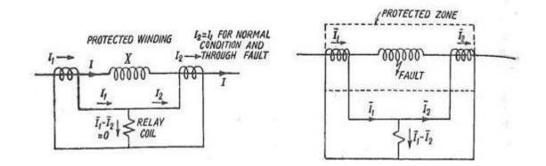
During normal condition and external fault the protection system is balanced and the CT's ratios are such that secondary currents are equal. These current circulate in pilot wires. The
