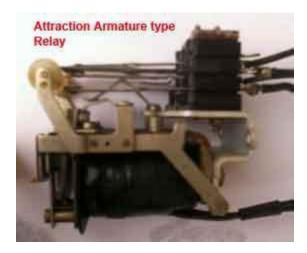
Hinged armature and plunger type constructions are most commonly used for these types of electromagnetic relays. Among these two constructional design, hinged armature type is more commonly used.
