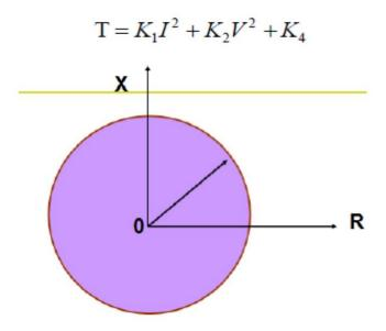
Considering K2 to be negative (as it produces the restraining torque) and neglecting the torque component due to spring, the equation represents a circle in the R-X plane.
