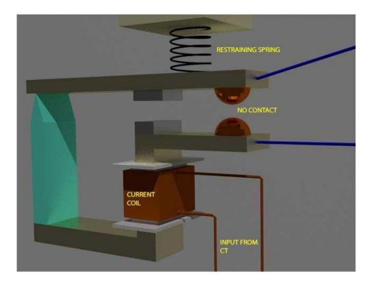
Here generally a magnetic core is wound by current coil. A piece of iron is so fitted by hinge support and restraining spring in the relay, that when there is not sufficient current in the coil, the NO contacts remain open. When current in the coil crosses a present value, the attractive force becomes sufficient to pull the iron piece towards the magnetic core and consequently the No contacts are closed.
